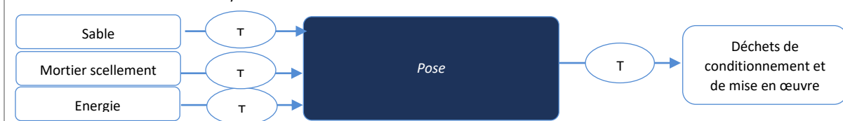
A5 – Processus de construction / Installation
